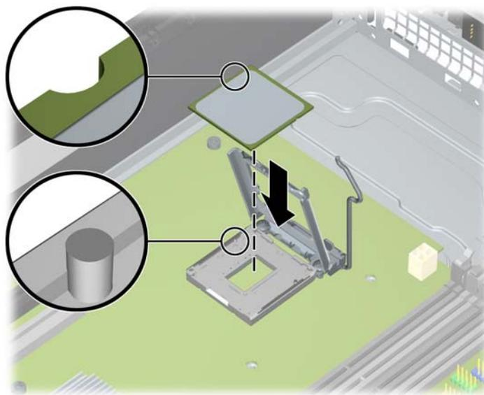
7. Close the CPU cover plate by lightly pressing down on the CPU cover plate while closing the socket lever.
