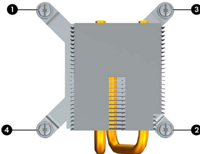
5. Disconnect the heatsink screws from the system board (1) as shown in the following figure.
