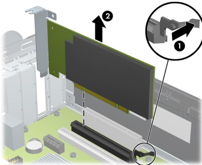
6. Install an expansion slot cover if you do not intend to replace the card.
