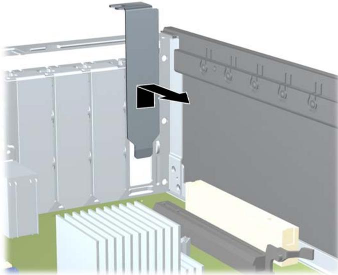
5. Angle the expansion card to insert it into the expansion card guide.
