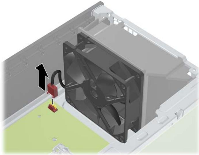
7. Remove the fan assembly by pushing in on the four release tabs on the front of the chassis (1), and then sliding the fan assembly into the chassis until you can lift it out.
