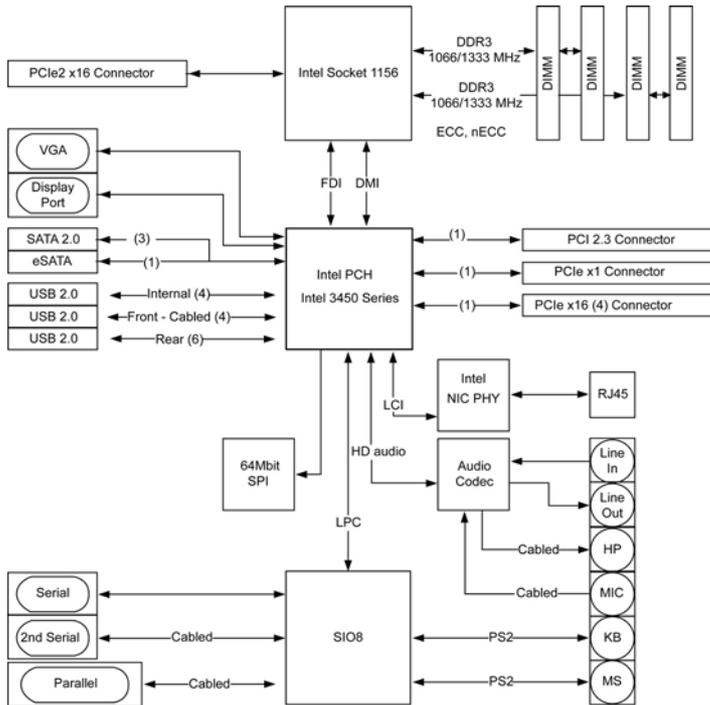
**NOTE:** The x1 and x16 designators describe the mechanical length of the slot. The number in parentheses lists the number of electrical PCIe lanes routed to the expansion slot. For example, x16(4) means that the expansion slot is mechanically a x16 length connector, with four PCIe lanes connected.
