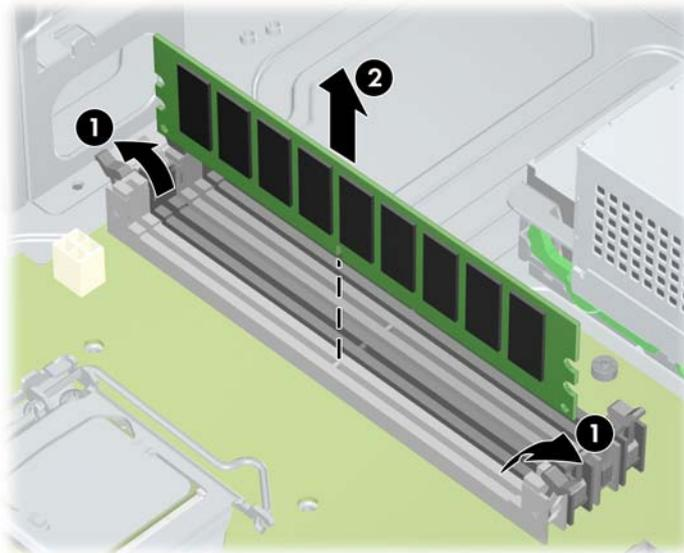
5. Lift the DIMM straight up (2) and out of the socket, then store the DIMM in an antistatic bag.
