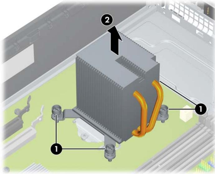
6. Before lifting the heatsink, gently twist the heatsink to break the thermal compound between the CPU and the heatsink.
