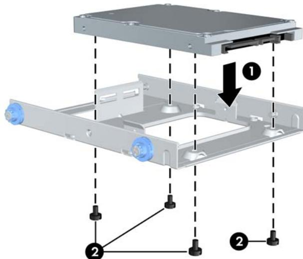
9. Align the guide screws with the slots on the chassis drive cage, press the hard drive down into the bay, then slide it back until it stops and locks in place.
