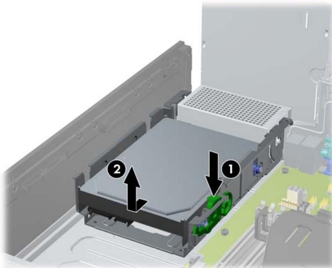
8. To install a new hard drive, the silver and blue isolation mounting guide screws from the old hard drive to the new hard drive.
